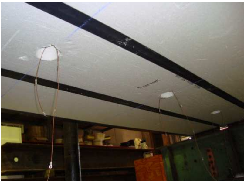
Figure 15. Displacement Transducer Attached to the Specimen
