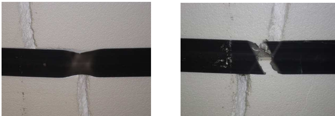
Figure 20. Furring Assembly Failure, "Necking" (left) and Fracture (right)
