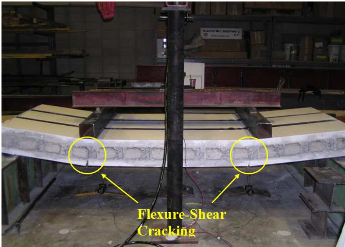
Figure 18. Flexural-Shear Cracking of the Specimen
