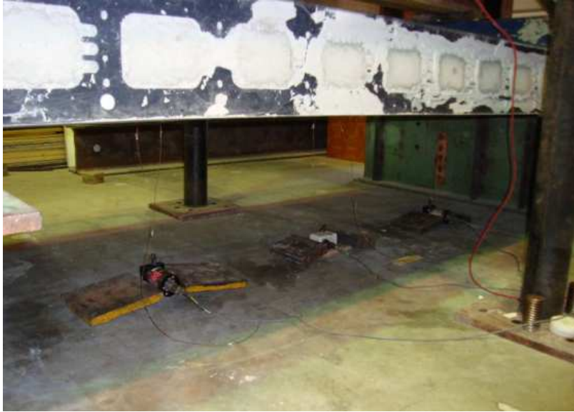
Figure 14. Displacement Transducer Placement
