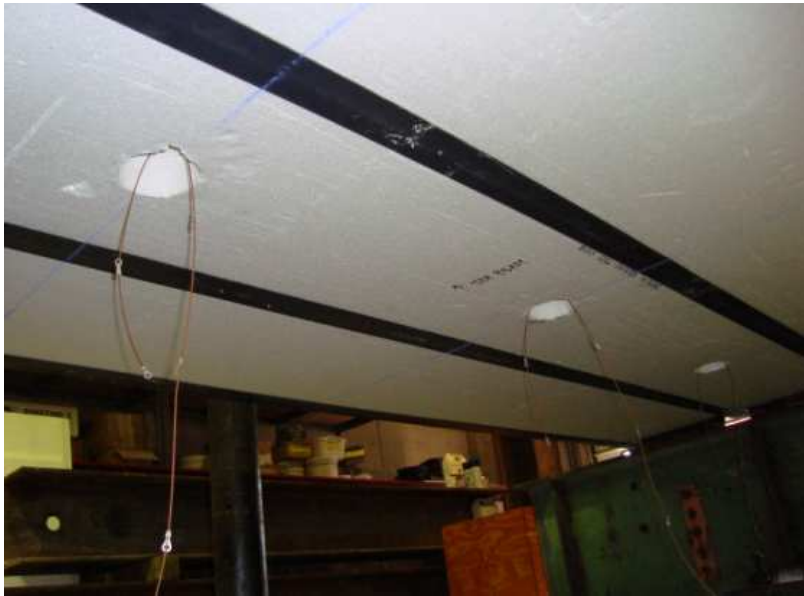
Figure 15. Displacement Transducer Attached to the Specimen
