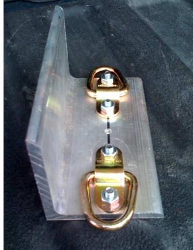
Figure 1. Fastener Pulling Apparatus
