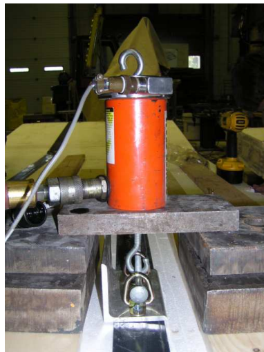
Figure 2. Fastener Pull-Out Testing Set-up
